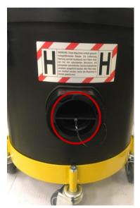
The container is equipped with a plug which is to be used during transport and whenever the machine is not operating.
