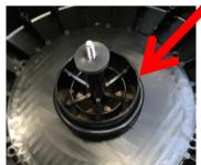
Pull a plastic bag (100 µm or the like) over the filter.
