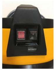
The automatic start/stop is activated with the black switch on the motor top. When the automatic start/stop is activated, the machine will not start when you push the red switch. The machine will not start until the hand tool connected is started.
