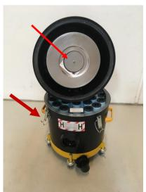
Loosen the four container clips of the motor top and remove the motor top. Place the motor top so that the filter is easily accessible.
