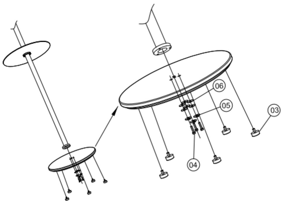
Step2: assemmble heater cross the pole and base.
